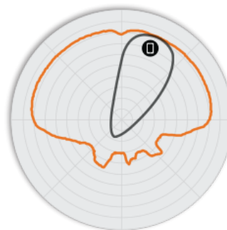
Figure 4. H510 2.4GHz Elevation Antenna Patterns
