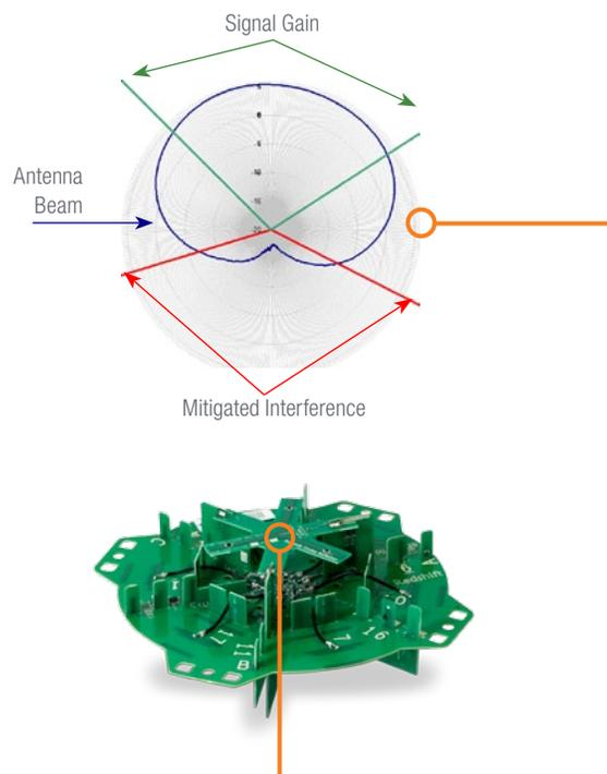
BeamFlex not only focuses RF energy only where it's needed but also mitigates interference coming from other directions. This ensures that the highest possible PHY rate is used and that the highest possible throughput is achieved for all clients.
